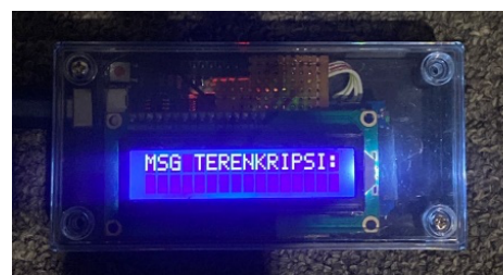
Gambar 7: Tampilan LED Saat Text Terenkripsi
