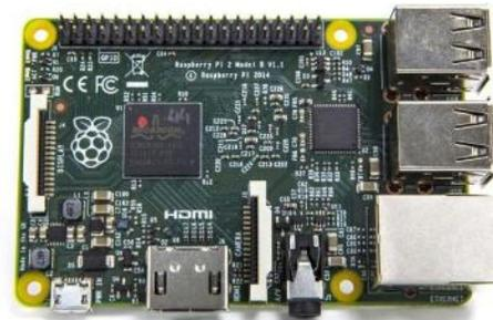
Gambar 2. Raspberry Pi 2 Board
